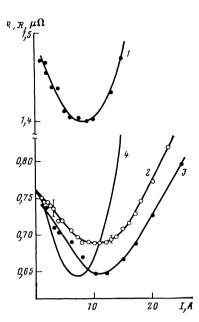
FIG. 4. Resistance (curves 1-3) and differential resistance (curve 4) of tungsten plates as a function of the current. 1) W3 plate, T = 1.5 K; 2, 3) W4 plate, T = 4.2 and 1.5 K; 4) W4 plate, T = 4.2 K.
