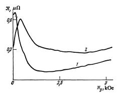
FIG. 1. Differential resistance of tungsten plate W1 in a longitudinal magnetic field, T=4.2 K. Curves 1 and 2 correspond to  $\mathcal{R}(I=0)\approx R_0$  and  $\mathcal{R}(I=7.5$  A), respectively.
