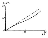
FIG. 3. Voltage-current characteristic of cadmium plate Cd1, T = 1.5 K. The dashed line shows the dependence  $U = R_0 \iota$ .
