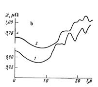
FIG. 7. Oscillations of the differential resistance as a function of the current. a) Plate W2, H = 0.1) T = 4.2 K; 2) T = 3.4 K; 3) T = 1.5 K; b) Plate W1, T = 4.2 K; 1) H = 0; 2)  $H = H_x = 20$  Oe.
