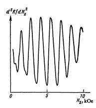
FIG. 2. Sondheimer oscillations in tungsten plate W1;  $H \parallel [100]$ , T = 4.2 K.
