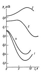
FIG. 6. Influence of an external magnetic field H on the differential resistance of tungsten plate W1 at T=4.2 K. 1) H=0; 2, 3)  $H=H_x=60$  Oe and 120 Oe, respectively; 4)  $H=H_v=100$  Oe.
