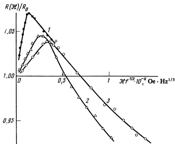
FIG. 2. Dependence  $R(H)/R_0$  for silver. Curve 1 corresponds to  $f = 1.75$  kHz, curve 2 to 23 kHz, and curve 3 to 98 kHz.  $T = 4.2$  K.
