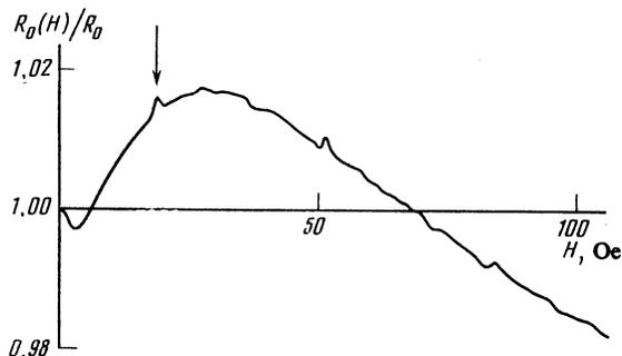
FIG. 3. Dependence of the linear surface resistance of tungsten (sample W1) on the static field  $(H) \parallel [100]$ ;  $H = 0.3$  Oe,  $f = 20$  kHz,  $T = 1.5$  K.
