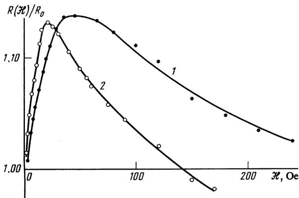
FIG. 6. Influence of temperature on the nonlinear surface resistance  $R(\mathcal{H})$  of tungsten (sample W3) obtained at  $f = 20$  kHz. Temperature (K): 1) 4.2; 2) 1.6.
