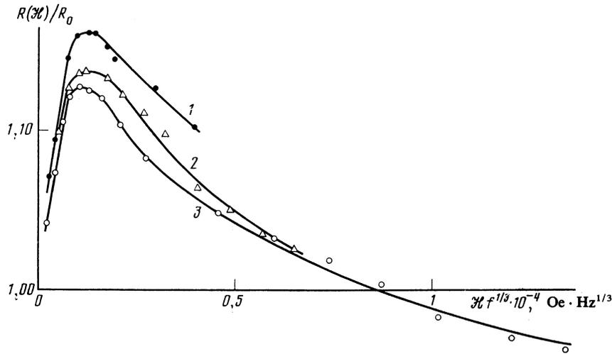
FIG. 5. Nonlinear surface resistance of tungsten (sample W3) at different frequencies. The alternating magnetic field is directed along the [110] axis. Frequency (kHz): 1) 1.8; 2) 20; 3) 98.
