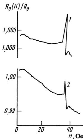
FIG. 4. Records of the rf size effect in tungsten (sample W3) obtained for  $H \parallel [110]$  and  $H = 0.3$  Oe at  $T = 4.2$  K for two values of the frequency:  $f = 20$  kHz (curve 1) and 98 kHz (curve 2).
