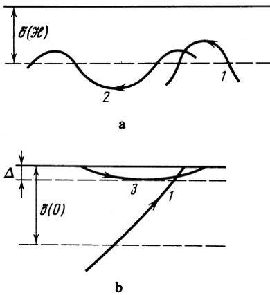
FIG. 7. Paths of "effective" electrons in a magnetic field of a wave in the skin layer: a) strong nonlinearity; b) weak nonlinearity; 1) untrapped electrons; 2) trapped electrons; 3) localized electrons.
