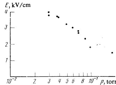
FIG. 3. Threshold field for the plasma-resonance discharge versus the pressure.
