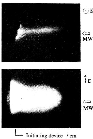
FIG. 2. Time-integrated photographs of the discharge.
