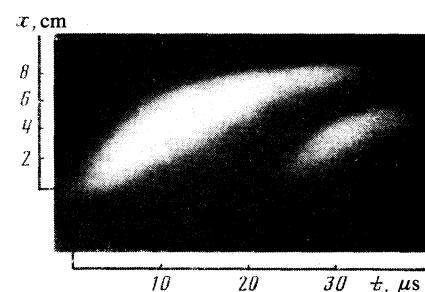
FIG. 4. "Photochronograms" (streak photos) of the discharge.
