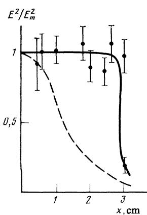
FIG. 6. Transverse field distribution in the focal region measured in the presence of the plasma (solid line) and in the absence of the plasma (dashed line).
