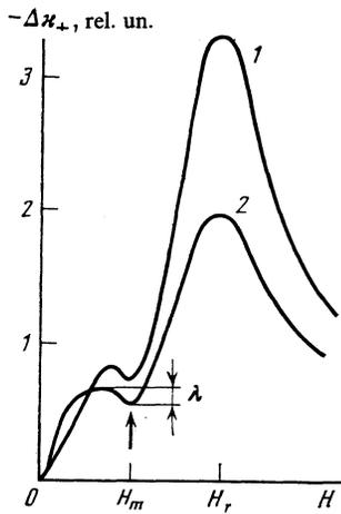
FIG. 2. Experimental plots of the change  $\Delta\kappa_+(H)$  of the thermal conductivity of CO gas in crossed fields.  $H_1 = 180$  kOe,  $f = 338$  kHz, and  $H_r = 1660 \pm 30$  Oe, 1)  $\nabla T \parallel \mathbf{H}$ ; 2)  $\nabla T \perp \mathbf{H}$ .
