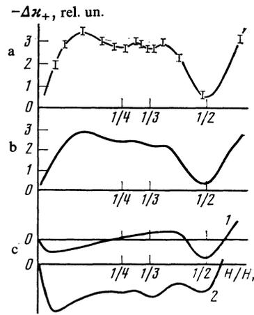
FIG. 4. Normalized experimental plots:  $\Delta\kappa_+(H/H_r)$ ,  $p = 30$  mTorr: a)  $f = 183$  kHz,  $H_1 = 130$  Oe; b)  $f = 338$  kHz,  $H_1 = 180$  Oe; c) theoretical curves for the models (see the text) with: 1)  $l_1 = 1$  and  $l_2 = 2$ ; 2)  $l_1 = 3$  and  $l_2 = 4$ .
