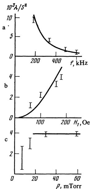
FIG. 3. Experimental plots for  $N_2$  at  $\nabla T \parallel \mathbf{H}$ : a) of  $\lambda/S^{\parallel}(f)$  at  $H_1 = 180$  Oe and  $p = 30$  mTorr; b) of  $\lambda/S^{\parallel}(H_1)$  at  $f = 338$  kHz and  $p = 30$  mTorr; c) of  $\lambda/S^{\parallel}(p)$  at  $f = 338$  kHz and  $H_1 = 180$  Oe. Solid curves—theoretical.
