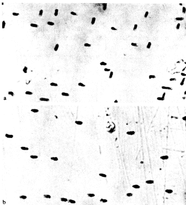
FIG. 2. Appearance of \alpha -particle tracks in a control sample (a) and in a sample exposed to a laser pulse (b).
