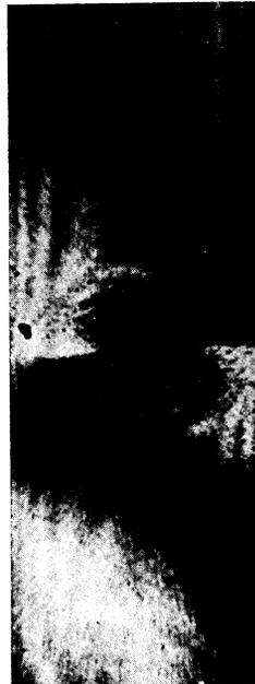
FIG. 2. Topographic section with an image of four closely spaced screw dislocations (the distance between dislocations is  $\approx 2\text{--}5 \mu\text{m}$ ). Crystal thickness of  $410 \mu\text{m}$ ; Mo  $K\alpha$  radiation; (660) reflection; dislocation axis parallel to the [110] direction;  $1/2[110]$  Burgers vector for each dislocation; (111) surface of the crystal.
