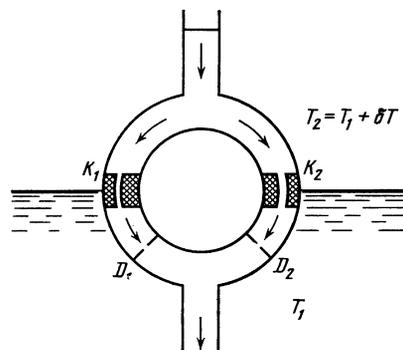
FIG. 3. Schematic form of apparatus for the observation quantum interference effects in helium II.  $K_1, K_2$ —capillaries;  $D_1, D_2$ —Josephson junctions.
