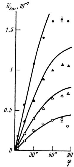
FIG. 3. Angular dependences of the second harmonic signal  $\tilde{u}_{2\omega}$  in the high-temperature phase ( $\Delta T = 4$  K) at  $u_{\omega} = 6 \times 10^{-7}$  for several values of the field:  $\bullet$ — $H = 4.5$  kOe;  $\blacktriangle$ — $H = 3$  kOe;  $\triangle$ — $H = 2$  kOe;  $\circ$ — $H = 1.4$  kOe.
