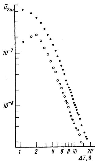
FIG. 5. Temperature dependences of the second harmonic signal  $\tilde{u}_{2\omega}$  in the high-temperature phase:  $u_\omega \approx 6 \times 10^{-6}$ ,  $\varphi = 45^\circ$ ; 1 || a: ○— $H = 2$  kOe, ●— $H = 4.5$  kOe.
