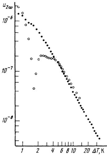
FIG. 2. Temperature dependences of the amplitude of the second harmonic near the spin-flip region at  $\mathbf{H} = 0$ ;  $\circ$ —low-temperature phase,  $\mathbf{I} \parallel c$ ;  $\bullet$ —high-temperature phase,  $\mathbf{I} \parallel a$ ;  $u_{\omega} \approx 3 \times 10^{-6}$ .
