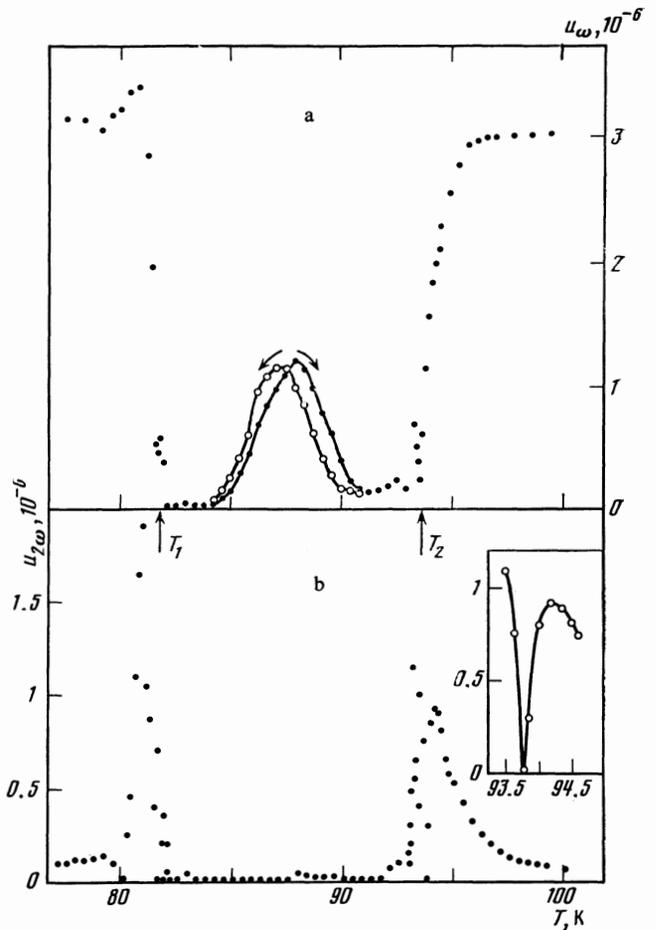
FIG. 1. Temperature dependences of the fundamental-frequency signal  $u_\omega$  passing through the sample (a) and the amplitude of the second-harmonic signal  $u_{2\omega}$  (b) at  $H = 0$ . The inset shows the region of transition  $T_2$  with tripled temperature scale.
