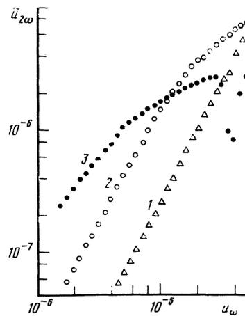
FIG. 6. Amplitude dependences of the strain  $\tilde{u}_{2\omega}$  in the high-temperature phase:  $H = 4.5$  kOe,  $\varphi = 45^\circ$ ,  $\Delta T = 5$  K, ○— $T = 1.7$  K, ●— $T = 0.2$  K.
