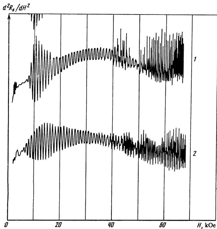
FIG. 2. Traces of oscillations of  $d^2R_s/dH^2$  as a function of magnetic field  $H$  for the case of symmetric excitation of the wave for the angles: 1)  $\theta \approx 0^\circ$ , 2)  $\theta \approx 5^\circ$ ;  $f = 3$  MHz.
