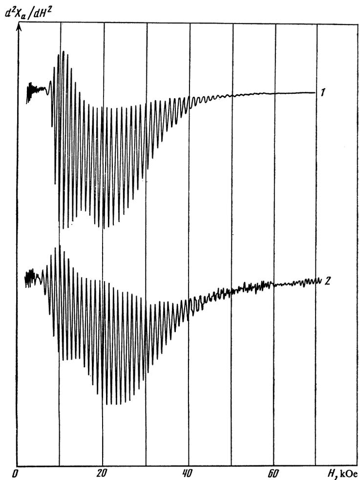
FIG. 3. Traces of oscillations of  $d^2X_a/dH^2$  as a function of magnetic field for the case of antisymmetric excitation of the wave: 1)  $\theta \approx 0^\circ$ , 2)  $\theta \approx 5^\circ$ ;  $f = 3$  MHz.
