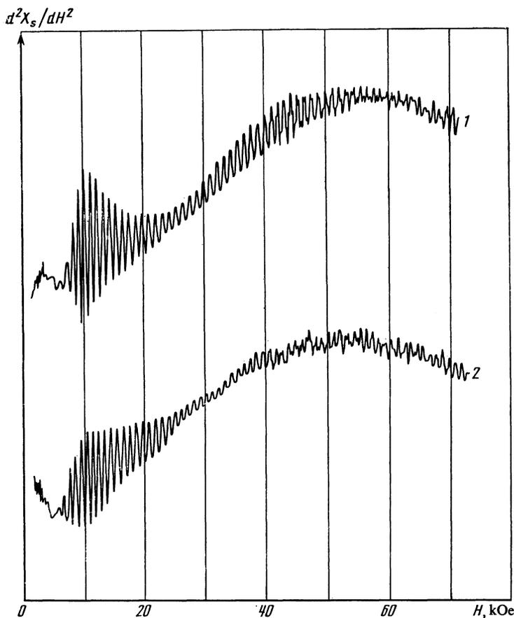
FIG. 4. Trace of oscillations of  $d^2X_s/dH^2$  as a function of magnetic field for the case of symmetric excitation of the wave: 1)  $\theta \approx 0$ , 2)  $\theta \approx 5^\circ$ ;  $f = 3$  MHz.
