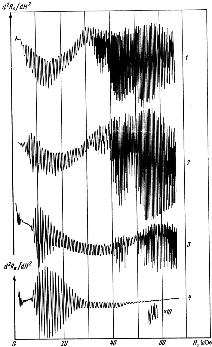
FIG. 1. Experimental traces of  $d^2R_s/dH^2$  and  $d^2R_a/dH^2$  for symmetric and antisymmetric excitation: 1)  $f = 0.58$  MHz; 2)  $f = 1$  MHz; 3,4)  $f = 3$  MHz;  $d = 0.186 \mu\text{m}$ ;  $\mathbf{H} \parallel \mathbf{C}_4$ ,  $T = 4.2$  K.
