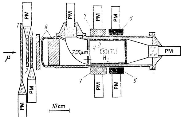
FIG. 2. Diagram of experimental setup: 1) counter that monitors the passage of the second meson; 2, 3, 4) monitoring counters; 5) vessel counter enclosing the working volume of the target; 6, 7) secondary-particle detectors with NaI and stilbene scintillators, respectively; 8) decelerating filter; PM) photomultiplier.
