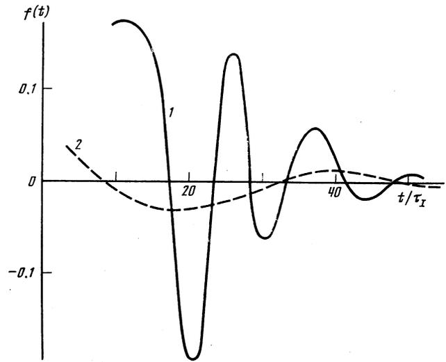
FIG. 1. The time dependence of the homogeneous magnetization of a ferromagnetic crystal:  $f(t) = (\tau_I/\tau) \bar{I}(t)/I_0$ . Curve 1)  $\omega_0 \tau_I = 0.5$ ,  $\tau_I/\tau = 0.1$ , curve 2)  $\omega_0 \tau_I = 1.5$ ,  $\tau_I/\tau = 0.01$ .
