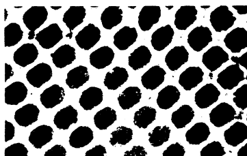
FIG. 5. Vortex lattice in NLC with \epsilon_d > 0 : magnification 250 \times ; U_x = 5 V, U_h = 20 V.
