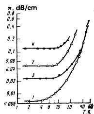
FIG. 3. Temperature dependence of the damping of longitudinal hypersound in lithium niobate along a threefold axis at a frequency of 3 GHz—(1) and (3), 9.4 GHz—(2) and (4); 1 and 2—with reversal ( $R = 44.8$  mm,  $L = 442$  mm,  $\varepsilon = -0.2$ ), 3 and 4—without reversal.
