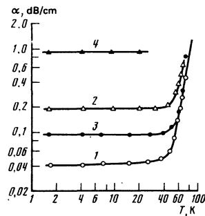
FIG. 4. Temperature dependence of the damping of longitudinal hypersound in sapphire along a threefold axis at a frequency of 3 GHz—(1) and (3), 9.4 GHz—(2) and (4); 1 and 2—with reversal ( $R = 44.8$  mm,  $L = 22.5$  mm,  $\varepsilon = -0.016$ ), 3 and 4—without reversal.
