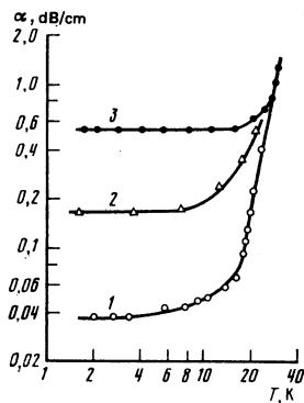
FIG. 5. Temperature dependence of the damping of longitudinal hypersound in quartz along threefold axis at a frequency of 3 GHz (1) and (3) and 4 GHz—(2); 1 and 2—with reversal ( $R = 119$  mm,  $L = 40$  mm,  $\epsilon = 0.26$ ), 3—without reversal.
