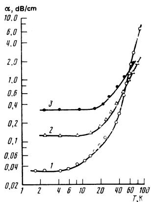
FIG. 6. Temperature dependence of the damping of longitudinal hypersound at a frequency of 3 GHz in lithium niobate along the normal to the plane of symmetry (1) and along the longitudinal normal, lying in the plane of symmetry of the crystal; 1—with reversal ( $R = 44.8$  mm,  $L = 16$  mm,  $\epsilon = 0.06$ ,  $\delta = -0.15$ ); 2—with reversal ( $R = 44.8$  mm,  $L = 3.4$  mm), 3—without reversal.
