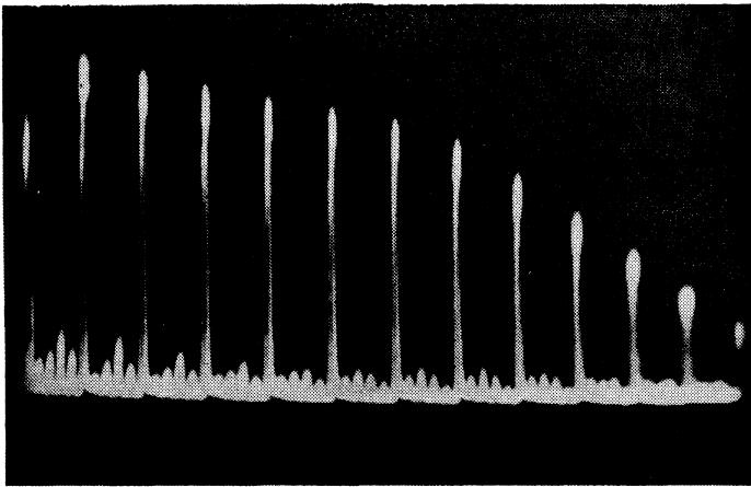
FIG. 2. Oscillogram of echoes of longitudinal hypersound in a sapphire crystal in the case of planar-spherical geometry of the reflecting surfaces. Every fifth echo is separated in amplitude.
