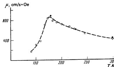
FIG. 3. Variation of the mobility of a DW of intermediate type, in a chemically polished specimen of TmFeO<sub>3</sub>, with temperature. The dark points denote the mobility determined from the slope of the  $V(H)$  curves; the light points, by the method of Rossol.
