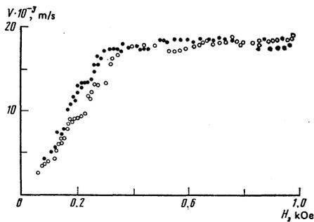
FIG. 4. Variation of the velocity of motion of Bloch and Néel walls, in a chemically polished specimen of  $\text{YFeO}_3$ , with the amplitude of a pulsed magnetic field. The light points denote the velocity of a Néel wall, the dark points that of a Bloch wall.
