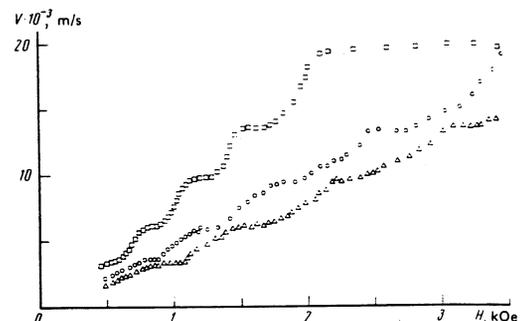
FIG. 1. Variation of the velocity of motion of a DW of the intermediate type, in a chemically polished specimen of  $\text{TmFeO}_3$ , with the amplitude of a pulsed magnetic field, at various temperatures:  $\Delta$ , 293 K;  $\circ$ , 227 K;  $\square$ , 178 K.
