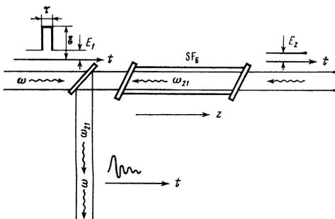
FIG. 2. Schematic representation of the observation of the resonant coherent transient process.
