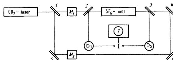
FIG. 1. Experimental arrangement:  $M_1$  and  $M_2$  are electro-optic light modulators;  $D_1$  and  $D_2$  are photodetectors; 7 is an oscilloscope; 1-6 are mirrors.
