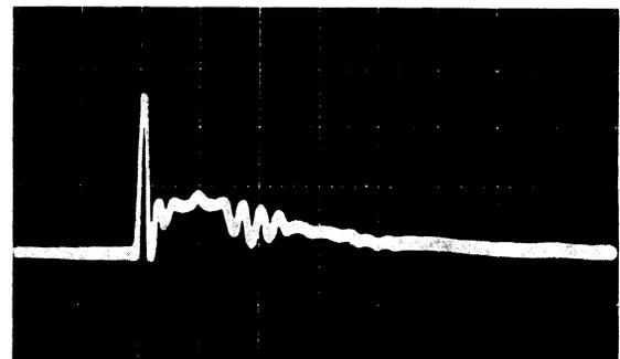
FIG. 5. Oscillogram of the RCTP signal for a line consisting of three components. One horizontal division represents 1  $\mu\text{sec}$ .
