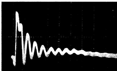
FIG. 3. Oscillogram of the RCTP signal. Each horizontal division represents  $1 \mu\text{sec}$ .
