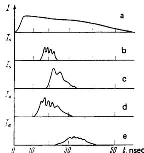
FIG. 2. Oscillograms of the exciting (a), Stokes (b, c), and anti-Stokes (d, e) pulses. The oscillograms b-e were obtained for different shots;  $p = 3 \text{ atm}$ ,  $W = 0.35 \text{ J}$ ,  $t_l = 3 \text{ nsec}$ .
