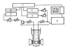
FIG. 2. Block diagram of spectrometer: 1) pulse supply unit, 2) modulator, 3)  $\omega_{ph}$  generator, 4)  $\omega_n$  generator, 5)  $2\omega_n$ generator, and 6) receiver.
