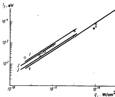
FIG. 3. Computed  $T_2(q_L)$  dependences for  $M_1 = 0.11$ ,  $A/Z = 3$  (the straight lines 2 and 3), 4 (1), and 2 (4), and a 50% (the straight lines 3 and 4) and 100% (the lines 1 and 2) laser-radiation power conversion into hydrodynamic energy flux.  $\circ$ )  $T_h$  values taken from Refs. 23 and 24;  $\bullet$ )  $E_{fi}/3Z$  values from Refs. 26 and 27 respectively;  $\Delta$ )  $E_{as}/3Z$  values from Ref. 13;  $\square$ )  $T_Z$  values.
