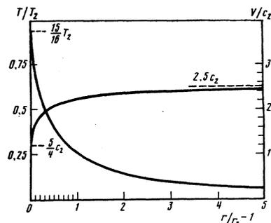
FIG. 2. The dependences  $T_e/T_2$  and  $V/c_2$  in the supercritical region.
