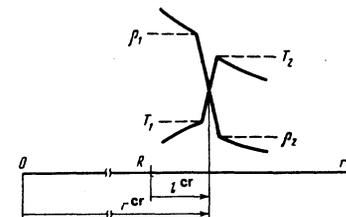
FIG. 1. Hydrodynamic "discontinuity" in the neighborhood of the critical point. The behavior of the quantities  $T_e$  and  $\rho$  at the discontinuity. The indices 1 and 2 denote the values of the quantities respectively to the left and right of the discontinuity.
