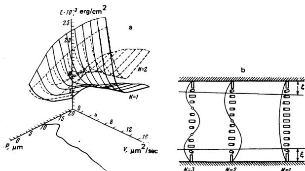
FIG. 2. Determination of the parameters of instability of plane flow. a—change of twist energy on transition from the first to the second Grandjean zone, at  $P=13 \mu\text{m}$  and  $V=2 \mu\text{m}^2/\text{sec}$ . b—schematic sketch of the distribution of molecules in the instability region. The curve in the  $PV$  plane is the projection of the spatial line of intersection of the energy surfaces for  $N=1$  and for  $N=2$ .
