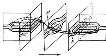
FIG. 4. Interaction of disclinations during the development of instability on lines of flow. For clarity, the figure has been turned  $90^\circ$  with respect to the preceding figure.
