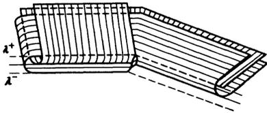
FIG. 5. Distortion of cholesteric layers on lines of disclinations during relaxation of instability.
