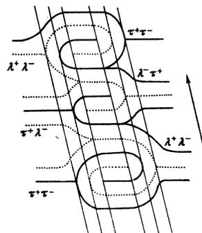
FIG. 3. Disclination model of the structure of lines of flow. The arrow shows the direction of the diffusion flow.
