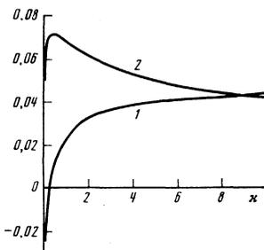
FIG. 3. Dependence on  $\kappa$  of the relative jumps of the speed (curve 1— $\Delta_1$ ) and of absorption (curve 2— $\Delta_2$ ) of the longitudinal sound at the critical angle  $\alpha_0$ .
