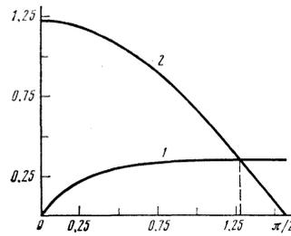
FIG. 1. Graphic solution of Eq. (4.12) at  $\kappa = 0.812$  ( $B = 1$ ); 1—the function  $[(\sin \varphi) / \kappa(\pi + \varphi)] \ln [\kappa(\pi + \varphi) / \sin \varphi]$ , 2—the plot of  $(1/\kappa) \cos \varphi$ .
