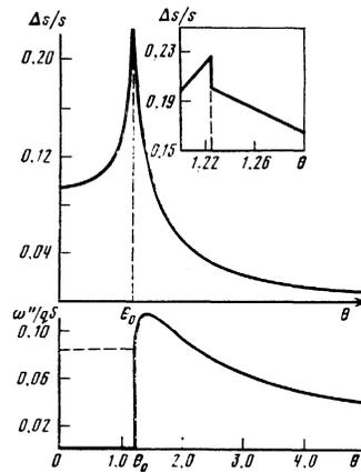
FIG. 4. Dependence of the change of the relative speed of sound  $\Delta s/s = (s(\alpha) - s)/s$  and of the relative absorption on  $\theta = \alpha v/s$  for an isotropic metal ( $B=1$ ); the inset shows the vicinity of the maximum.
