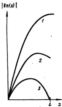
FIG. 2. Behavior of the perturbations  $\delta n_x(z)$  and  $\delta n_z(z)$  of the director in a cell of thickness  $L$ , in relative units, for various values of the parameter  $\xi$ : 1,  $\xi = 0$ ; 2,  $\xi = 1$ ; 3,  $\xi = \infty$ .
