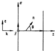
FIG. 3. Schematic diagram of self-focusing of light in a cell with NLC, with distorted director orientation. In the plane  $z = 0$ , the director  $\mathbf{n}(\mathbf{r})$  is oriented along the  $x$  axis; in the plane  $z = L$ , along the  $z$  axis.
