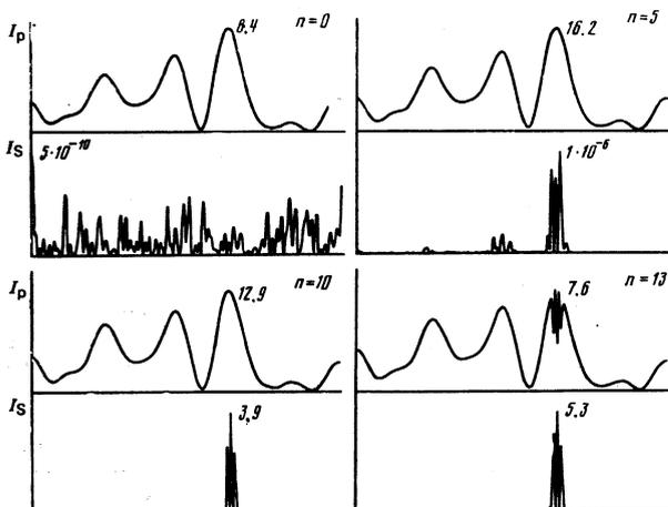
FIG. 2. Computer oscillograms of generation at  $m_s \gg m_p$ . The numbers next to the maxima of each curve indicates the value of this maximum in units of  $I_p^{st}$ . The numbers next to the maxima of each curve indicates the value of this maximum in units of  $I_s^{st}$ . The laser parameters are:  $\eta = 7$ ,  $l = 70$  m,  $\delta = 400$ ,  $m_s = 60$ ,  $m_p = 6$ .
