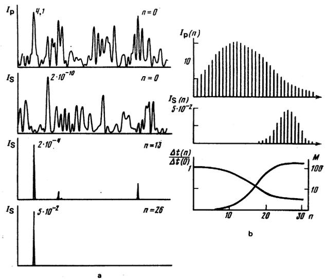
FIG. 3. Linear regime of RFL lasing. The structure of the pump radiation is shown only for  $n = 0$ . The laser parameters are:  $\eta = 4$ ,  $l = 70$  m,  $\delta = 400$ ,  $m_s = m_p = 35$ .
