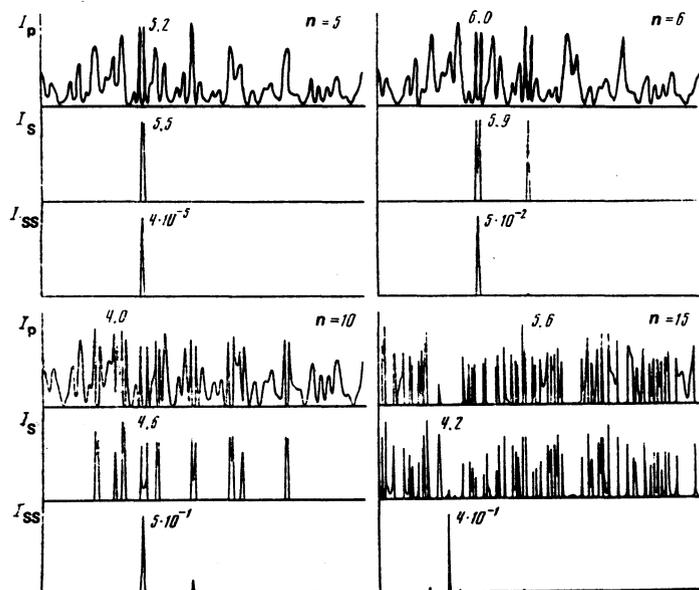
FIG. 7. Generation of the second Stokes component. Randomization of the time structure of the first Stokes component. The laser parameters are:  $\eta = 10$ ,  $l = 70$  m,  $\delta = 3000$ ,  $m_{ss} = \eta_s = m_p = 35$ .
