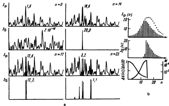
FIG. 4. Saturation of Raman gain. In the upper plot on the right the dashed curve shows the intensities of the maximum fluctuation bursts of the pump in the absence of Raman lasing ( $g=0$ ). The laser parameters are  $\eta=5$ ,  $l=70$  m,  $\delta=400$ ,  $m_s = m_p = 35$ .
