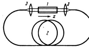
FIG. 1. Optical diagram of RFL: 1—active medium, 2—optical fiber, 3—matching lenses.
