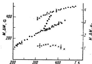
FIG. 2. Temperature variation of the magnetization of  $\text{DyCo}_{5.3}$  in zero external field. The triangles and circles denote the same values of magnetization as in Fig. 1. Squares: magnetization along an easy direction located at an angle to the hexagonal axis. Crosses: difference of magnetizations along the hexagonal axis and in the basal plane.
