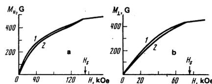
FIG. 4. Experimental (1) and theoretical (2) field dependences of the magnetization of  $DyCo_{5.3}$  along the hard direction: a)  $T = 320$  K, field directed along the hexagonal axis; b)  $T = 400$  K, field directed in the basal plane.
