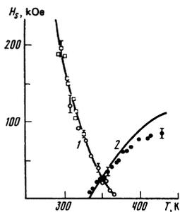
FIG. 3. Experimental (symbols) and theoretical (solid lines) temperature variations of the saturation field of  $\text{DyCo}_{5.3}$  along the hexagonal axis (1) and in the basal plane (2). Circles, from measurements of the field-dependence curves of the magnetization; squares, from magnetostriction measurements.
