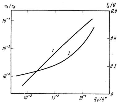
FIG. 1. Velocity of the front (1) and temperature on the phase boundary (2) in stationary evaporation.
