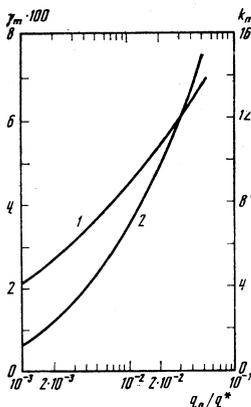
FIG. 3. Maximum instability growth rate (2) and corresponding value of the wave number (1) as a function of the radiation intensity.
