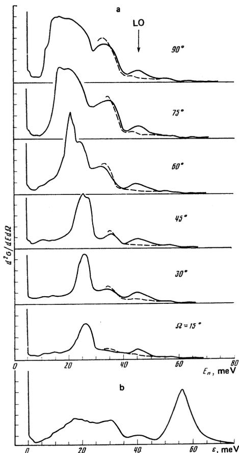
FIG. 1. Spectra of the cross sections for scattering of cold neutrons by the investigated Cu-Be alloys: a)  $\alpha$ -solution,  $c = 0.042$ , the dashed line shows the part of the spectrum of scattering by pure copper; b)  $\alpha$  + intermetallide CuBe,  $c = 0.27$ , angle  $\Omega = 90^\circ$ .
