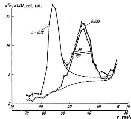
FIG. 7. Spectral distributions of the oscillations due to Be atoms in one-phase (○) and two-phase (●) Cu-Be samples. The widths of the LO at half-height are given in microseconds.  $N$  is the number of the time-analyzer channel.
