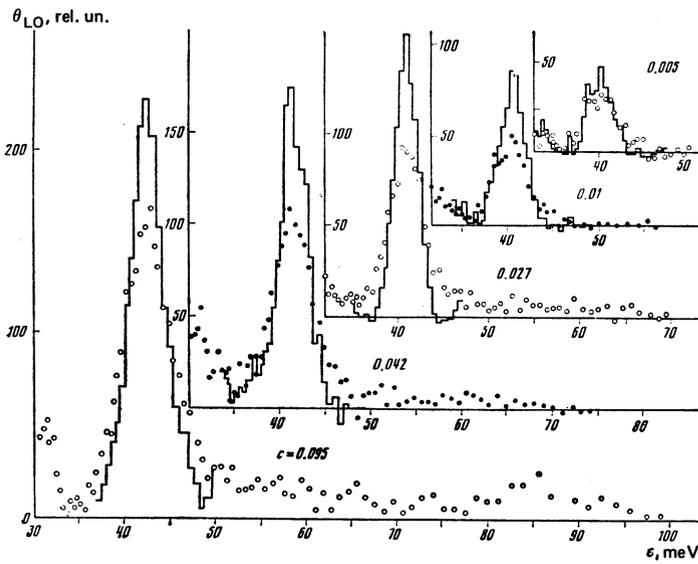
FIG. 2. Distribution function  $\Theta_{LO}(\epsilon)$  for different Be concentrations; points—experiment, histograms—reconstructed spectra.
