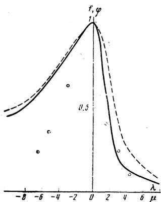
FIG. 3. Radiative-collision line shape in the weak-field approximation. Solid curve—the function  $f(\lambda)$ , dashed—the function  $\varphi(\mu)$ , points—experimental.
