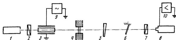
FIG. 2. Apparatus for measurements of small changes in the birefringence: 1) helium–neon laser; 2) polarizer; 3) light modulator; 4) sample; 5) quartz wedge; 6) Berek compensator; 7) analyzer; 8) photomultiplier; 9) oscillator; 10) measuring narrow-band amplifier.
