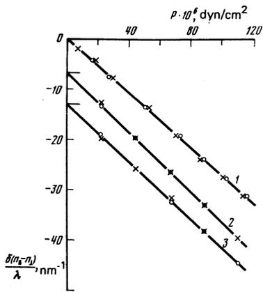
FIG. 3. Typical results of measurements of the piezoelectric effect in an  $\text{MnF}_2$  single crystal (sample No. 3, pressure along [110], light along [110]): 1) at helium temperatures (approximately 2 °K); 2) at nitrogen temperatures (approximately 55 °K); 3) at room temperature (approximately 295 °K). The circles were obtained by increasing the pressure and the crosses by reducing it.
