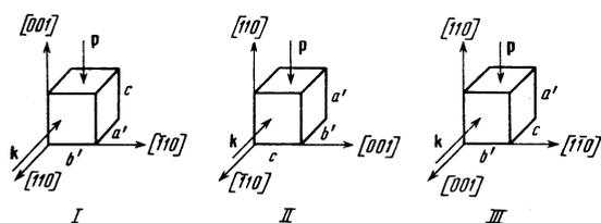
FIG. 4. Experimental geometries used to measure the piezoelectric effect.
