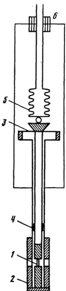
FIG. 1. Principal parts of the apparatus used to apply pressures: 1) sample between copper pistons; 2) thick-walled copper tube with windows; 3) membrane; 4) Teflon ring; 5) bellows; 6) guide for vertical motion of bellows.
