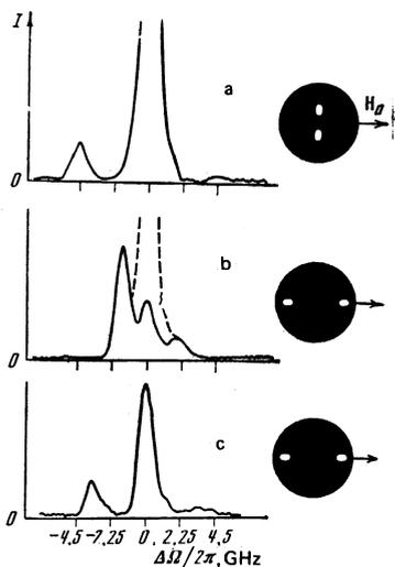
FIG. 4. Spectrum of scattered light at various  $H_0$  and  $\theta'_k$ : a)  $H_0 \approx H_{oc}$ ,  $\theta'_k \approx 90^\circ$ ; b)  $H_0 = 675 \text{ Oe}$ ,  $\theta'_k = 0$  (the dotted curve shows the spectrum when the analyzer is uncrossed by  $\pm 1^\circ$ ); c)  $H_0 = 1350 \text{ Oe}$ ,  $\theta'_k \approx 0$ . To the right of the figure are shown the diaphragms  $D_1$  (Fig. 1) used to obtain curves a-c.
