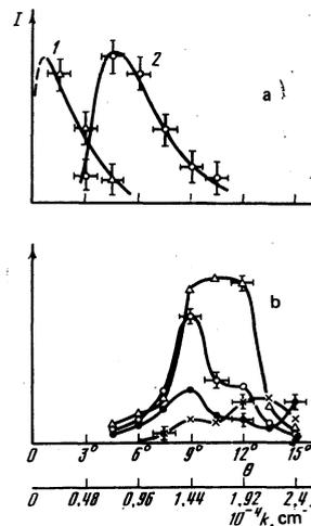
FIG. 3. Variation of the pulse component of the intensity  $I$  (in relative units) of the scattered light with scattering angle  $\theta$ , for fixed  $H_0$  and  $\theta'_k$ : a)  $H_0 \approx H_{0c} = 1050$  Oe,  $\theta'_k = 90^\circ$  (curves 1 and 2 correspond to two crystallographically equivalent positions of the specimen); b)  $\theta'_k \approx 0$ ,  $\bullet$ )  $H_0 = 549$  Oe,  $\Delta$ )  $H_0 = 758$  Oe,  $\odot$ )  $H_0 = 675$  Oe,  $\times$ )  $H_0 = 1350$  Oe.
