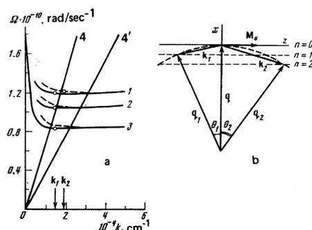
FIG. 8. a) Lower bounds of spin-wave spectrum ( $\theta'_k = 0$ ) in a thin plate of YIG at various values of  $H_0$ : 1)  $H_0 = 758 \text{ Oe}$ ; 2)  $H_0 = 675 \text{ Oe}$ ; 3)  $H_0 = 549 \text{ Oe}$ ; 4 and 4') the straight lines for elastic waves. The points denote experimental values corresponding to the scattering maxima at  $\theta'_k \approx 0$  (Fig. 3b) and to spectra of the type represented in Fig. 4b. b) Geometry of light scattering by quasiparticles with  $\theta'_k = 0$ .
