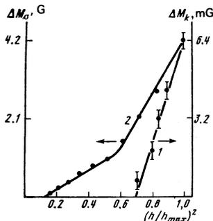
FIG. 5. Variation of the pulsed changes of magnetization of the crystal with pumping power. Curve 1, the change caused by production of magnons with  $\theta_k' = 90^\circ$ , satisfying the conditions for scattering of light. Curve 2, the change caused by all nonequilibrium magnons. External field  $H_0 \approx H_{0c}$ .
