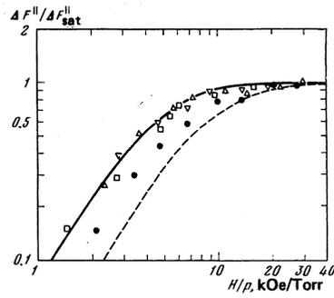
FIG. 3. The component of the TMF in N<sub>2</sub> normal to the surface vs H/p. The full curve and the open experimental points are the same as in Fig. 2 (r/L ≈ 1). The dashed curve represents Eq. (4.5) and the theory of Ref. 6. The black circles are experimental points measured with the disk shifted to such a position that r/L<sub>min</sub> ≈ 3.5 (Ref. 3).
