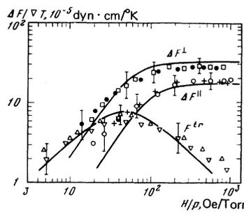
FIG. 1. The TMF in NO vs  $H/p$ . The experimental points were taken from Ref. 4 and were measured at various gas pressures for which  $\bar{l}/r \sim 0.1$ : The points  $\square$ ,  $\circ$ ,  $\Delta$ , and  $+$  were measured with an aluminum disk, and the points  $\nabla$  and  $\triangle$ , with a paper disk.
