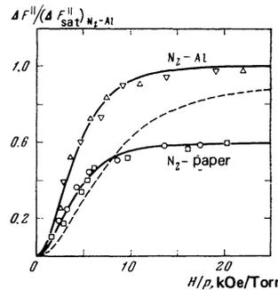
FIG. 2. The TMF on aluminum and paper surfaces in  $N_2$  vs  $H/p$ . The full curves represent Eq. (4.4) with  $c_3/c_1 = 0.7$  for aluminum and  $c_3 = 0$  for paper. The experimental points were taken from Ref. 3 and were measured at various gas pressures for which  $\bar{l}/r \sim 0.1$ . The dashed curve represents the theory of Ref. 6.
