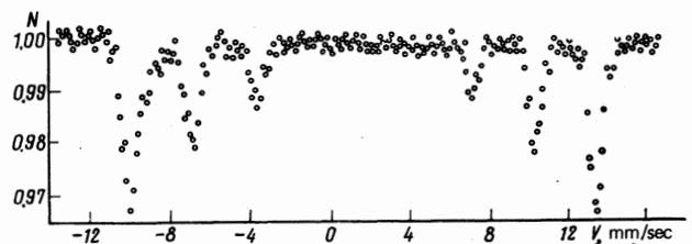
FIG. 1. Mössbauer resonance absorption spectrum of  $^{119}\text{Sn}$  in  $\text{Fe}_3\text{Ge}$  at 77° K.
