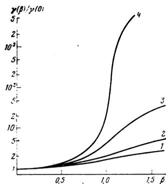
FIG. 2. The kinematic friction coefficient  $\gamma(\beta)$  referred to the value  $\gamma(0)$  vs. the drop velocity at various temperatures. Values of the parameter  $\xi = T_0/T$ : 1)  $\xi = 3$ , 2) 6, 3) 10, 4) 30.
