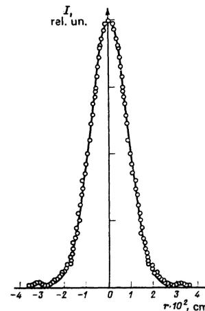
FIG. 2. Distribution of the intensity in a transverse cross section through a laser beam at the entry to a nonlinear medium: the points are the experimental results and the continuous curve is a Gaussian distribution.
