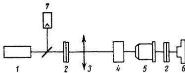
FIG. 3. Experimental setup: 1) laser; 2) neutral filters; 3) lens; 4) sample; 5) microscope; 6) photographic camera; 7) calorimeter.
