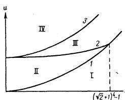
FIG. 2. Limiting velocities of magnetic moment waves of different types: 1)  $u = u_-(\epsilon)$ ; 2)  $u = [u_+^2(\epsilon) - u_-^2(\epsilon)]^{1/2}$ ; 3)  $u = u_+(\epsilon)$ .
