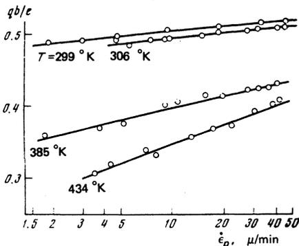
FIG. 2. Dependences of the dislocation charge  $qb/e = f$  in ZnSe on the deformation rate.
