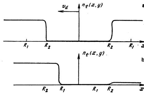
FIG. 5. Schematic diagram illustrating the solution of Eq. (8): (a) case  $R_1 > R_2$ ; (b) case  $R_1 < R_2$ .
