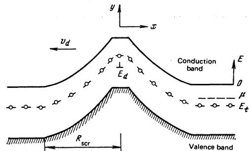
FIG. 1. Schematic representation of the bending of the allowed energy bands near a dislocation and the coordinate system adopted in calculations.
