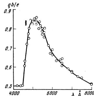
FIG. 4. Spectral dependence of the dislocation charge in ZnSe on the wavelength of incident light;  $T = 295$  K,  $\epsilon_p = 10 \mu/\text{min}$ .
