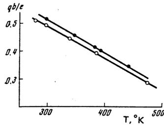
FIG. 3. Temperature dependences of the dislocation charge  $qb/e = f$  in ZnSe for two samples deformed at a rate  $\epsilon_p = 10 \mu/\text{min}$ .
