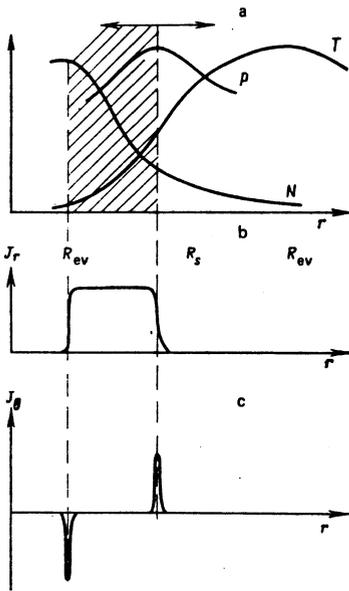
FIG. 1. Radial distributions of the temperature, pressure, and density (a) and of the radial (b) and angular (c) components of the currents near the front of the thermal wave. The arrows indicate the plasma motion direction. The shaded area is the instability zone,  $R_{ev}$  is the evaporation boundary,  $R_s$  is the Jouguet point, and  $R_{cr}$  is the critical radius.
