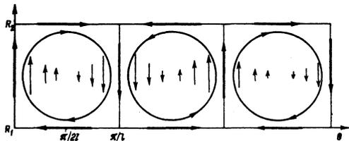
FIG. 2. Angular distribution of the currents in the instability zone for axially symmetrical perturbations.
