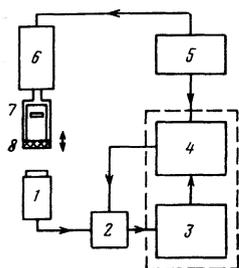
FIG. 1. Block diagram of current spectrometer: 1—NaI(Tl) crystal with FEU-13 photomultiplier, 2—integrator, 3—amplitude to digital converter (ADC), 4—time block of LP-4050 analyzer, 5—NGPK-3 generator, 6—vibrator, 7—source, 8—absorber.
