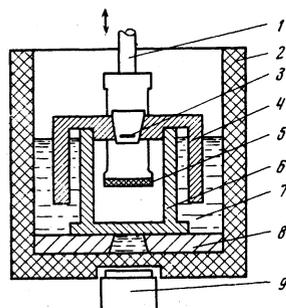
FIG. 2. Cooling system for source and absorber: 1—vibrator rod, 2—foam plastic, 3—source, 4—source holder, 5—absorber, 6—vessel, 7—liquid nitrogen, 8—collimator, 9—detector.
