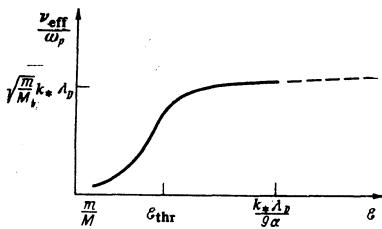
FIG. 5. Effective collision frequency as function of the pump amplitude in a non-isothermal plasma when the conversion due to short-wavelength sound is important ( $\mathcal{E} = E_0^2/8\pi n_0 T$ ).
