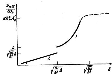
FIG. 7. Effective collision frequency in the case when the frequency "mismatch" of the pumping frequency is larger than the plasma frequency:  $\Delta > m/M$ .
