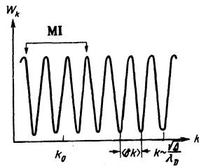
FIG. 6. Spectral transfer of plasma oscillations in the long-wavelength region according to weak turbulence and occurrence of the modulational instability (MI) at large "mismatches"  $\Delta > \Delta_0$ .
