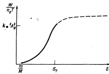
FIG. 3. Plasma noise energy as function of pump amplitude ( $W/n_0 T = \nu_{\text{eff}}/\alpha \omega_p$ ,  $\mathcal{E} = E_0^2/8\pi n_0 T$ ,  $\mathcal{E}_T = (m/M)^{1/2} k_* \lambda_D / \alpha$ ).
