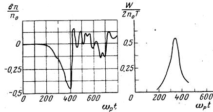
FIG. 4. Density variation and electrical field amplitude at the center of a caviton as functions of time in a numerical experiment.<sup>[12]</sup> When  $\omega_p t \sim 400$  the energy of the Langmuir field is damped and then the caviton becomes a source for short-wavelength sound oscillations.
