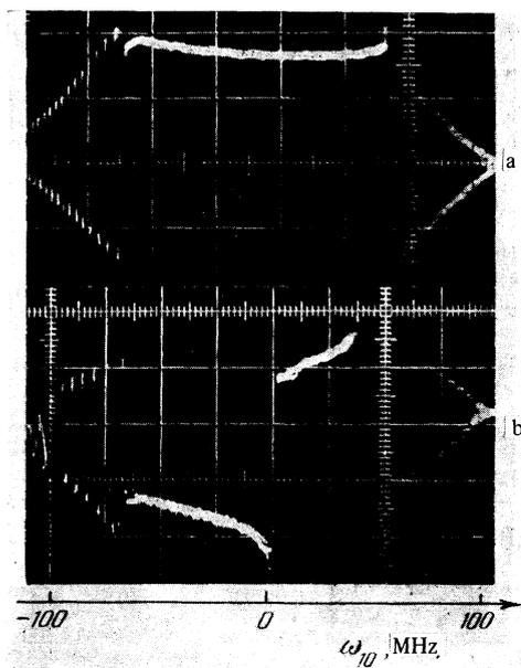
FIG. 3. Oscillograms of the beat signal as a function of the detuning  $\omega_{10}$  for the neon transition  $2s_2-2p_1$  at  $\Omega_{12} = \text{const}$ ,  $\omega_{10} = \omega_{12}/2$  for a)  $\psi = 0$  and b)  $\psi = \pi/2$ .
