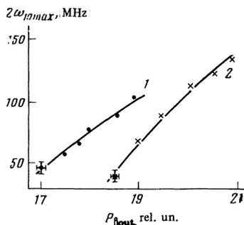
FIG. 2. Dependence of the locking region  $2\omega_{10\max}$  on the radiation output power  $P_{\text{out}}$  for the neon transition  $3s_2-3p_2$  at constant  $\Omega_{12}$  and pressures  $p=2.4$  Torr (curve 1) and  $p=1.7$  Torr (curve 2).
