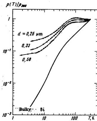
FIG. 1. Reduced temperature dependences of the resistivity of bulk Bi (basal plane)<sup>[8]</sup> and of cylindrical single crystals with different diameters  $d$ .
