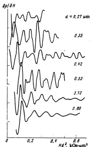
FIG. 5. Size-effect oscillations on the derivative of the longitudinal magnetoresistance as functions of the quantity  $Hd^2$  for cylindrical Bi single crystals with different diameters at  $T = 4.2$  K (the monotonic component is suppressed). For convenience in the analysis, the curves are shifted vertically by arbitrary amounts.
