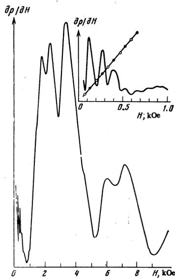
FIG. 4. Field dependence of the magnetoresistance derivative of a sample with  $d = 0.8 \mu\text{m}$  at  $T = 4.2 \text{ K}$ . The magnetic field is directed along the bisector (angle between  $H$  and  $J$  is  $19.5^\circ$ ). The insert shows the initial section of the curve in an enlarged scale and the dependence of the number of the extrema  $n$  on the plot of  $\partial\rho/\partial H = f(H)$  against the field  $H$ .
