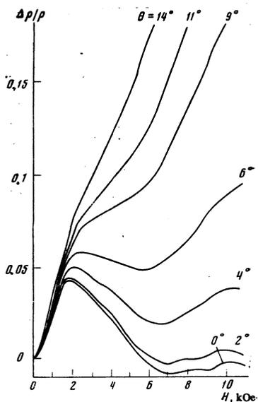
FIG. 2. Field dependences of the magnetoresistance of a cylindrical single crystal of Bi of  $0.76 \mu\text{m}$  diameter at  $T = 4.2 \text{ K}$  and at different orientations of the magnetic field  $H$  relative to the cylinder axis ( $\theta = 0$  at  $H \parallel J$ ).
