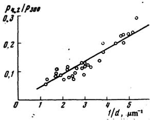
FIG. 6. Relative resistivity ( $T=4.2$  K) of cylindrical Bi single crystals vs. the reciprocal diameter.
