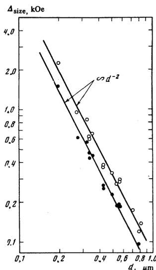
FIG. 9. Dependences of the periods of the size-effect oscillations of the longitudinal magnetoresistance on the diameter for cylindrical Bi single crystals.
