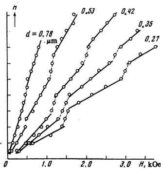
FIG 8. Dependence of the number of the extrema of the size-effect oscillations of the derivative  $\partial\rho/\partial H$  of the longitudinal magnetoresistance on the magnetic field for samples with different diameters.
