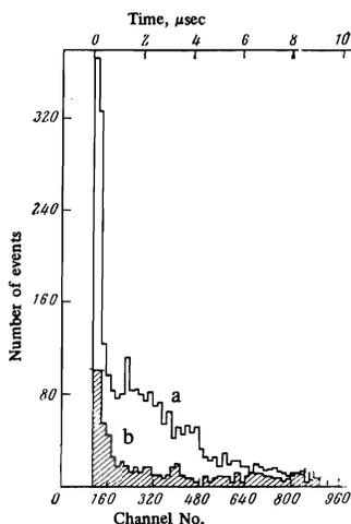
FIG. 2. Temporal spectra of events registered by  $\gamma$  detectors in anticoincidences with the counter 5 ( $\gamma_5$ ): a) run A  $H_2 + D_2$  mixture; b) Data of run B (He) normalized to the number of stopped muons in run A. The abscissas represent the time of the  $\gamma$  quantum measured from the time of stopping of the muon, while the ordinates represent the number of events in a time interval 0.189  $\mu$ sec.
