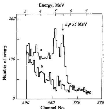
FIG. 3. Amplitude distributions of events registered by  $\gamma$  detectors in anticoincidence with counter 5: a) run A, b) normalized data of run B. The ordinates represent the number of events in a 0.092-MeV interval.
