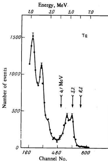
FIG. 4. Amplitude distribution of events registered by  $\gamma$  detectors in experiment I after subtracting the normalized of experiment II. The arrows indicate the position of the photopeak of the  $K_{\alpha}$  line of the  $Ta\mu$  atom and the limits of the range in which the events were reduced.
