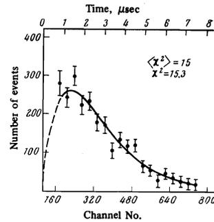
FIG. 5. Temporal distribution of  $\gamma$  quanta from the fusion reaction in the mesic molecule  $pd\mu$  (the normalized background was subtracted). Ordinates—number of events in  $0.378 \mu\text{sec}$  interval. Solid line—calculated curve.
