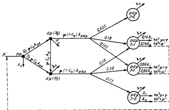
FIG. 1. Diagram of the processes occurring in the  $H_2 + D_2$  mixture after the stopping of a  $\mu^-$  meson.
