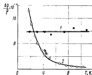
FIG. 5. Temperature dependence of the magnetoresistance for a crystalline (curve 1) and amorphous (curve 2) ytterbium film of thickness 110 Å;  $H \approx 16$  kOe.
