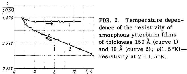
FIG. 2. Temperature dependence of the resistivity of amorphous ytterbium films of thickness 150 Å (curve 1) and 30 Å (curve 2);  $\rho(1.5^\circ\text{K})$ —resistivity at  $T = 1.5^\circ\text{K}$ .
