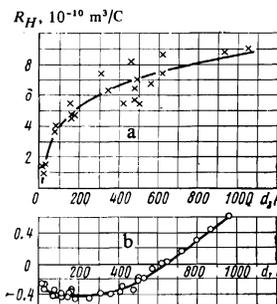
FIG. 7. Dependence of the Hall coefficient of the thickness of crystalline (Fig. a) and amorphous (b) ytterbium films.
