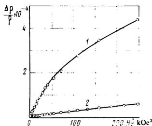
FIG. 3. Change of the resistivity of ytterbium film  $\sim 110$  Å thick in a magnetic field at the following temperatures: 1— $4.2^\circ\text{K}$ , 2— $10.3^\circ\text{K}$ ;  $\Delta\rho = \rho_H - \rho$ ,  $\rho_H$  is the resistivity in a magnetic field  $H$ ,  $\rho$  is the resistivity in the absence of a magnetic field.
