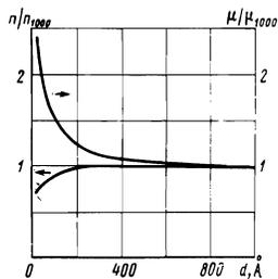
FIG. 8. Dependence of the number and mobility of the electrons (holes) on the thickness of amorphous ytterbium films;  $n_{1000} = 1.85 \times 10^{20} \text{ cm}^{-3}$  and  $\mu_{1000} = 1.4 \times 10^{-2} \text{ m}^2/\text{V}\cdot\text{sec}$  are the concentration and mobility of the electrons (holes) in amorphous films  $\sim 1000 \text{ \AA}$  thick.
