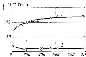
FIG. 1. Dependence of the resistivity of amorphous (curve 1) and crystalline (curve 2) ytterbium films on their thickness at  $T = 4.2^\circ\text{K}$ .
