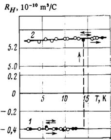
FIG. 6. Variation of the Hall coefficient with temperature for an ytterbium film 150 Å thick; 1—amorphous state, 2—crystalline state; ●—heating, ○—cooling.
