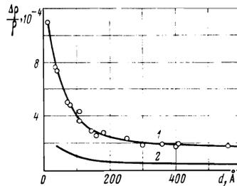
FIG. 4. Dependence of the magnetoresistance of amorphous ytterbium films on their thickness at  $T = 4.2^\circ\text{K}$ ; curve 1— $H \approx 16$  kOe, 2— $H \approx 4.5$  kOe.
