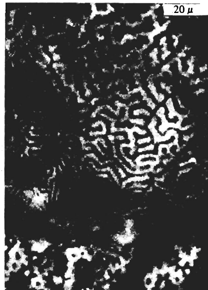
FIG. 4. Picture of the domain structure of a polycrystalline sample of \text{UCo}_{5.3} , displayed with the aid of the magneto-optical Kerr effect.
