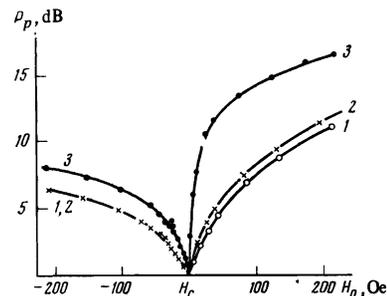
FIG. 1. Dependence of the threshold of parametric-instability excitation threshold on the constant magnetic field  $H_0$  in the case of parallel pumping  $P_p$ . Curves 1, 2, and 3 correspond to YIG spheres 1.02, 0.52, and 0.18 mm in diameter. The absolute value of the threshold field at the point  $H_c$  amounts to 0.27 Oe for curves 1 and 2 and 0.34 Oe for curve 3;  $H_0 \parallel [111]$ .
