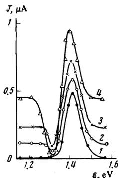
FIG. 4. Spectral dependence of the photocurrent  $J$  on the energy in the presence of constant monochromatic background illumination ( $\lambda = 8800$  Å) of intensity  $I_{\text{thr}}$  ( $U_{\text{thr}}/I_0$  is equal to zero (curve 1), 0.05 (curve 2), 0.125 (curve 3), and 0.25 (curve 4)). Sample  $\text{CdCr}_2\text{Se}_4$  (0.037% Ga). Field  $E \sim 50$  V,  $I_0 \sim 10^{-2}$  W/cm<sup>2</sup>,  $T = 77$  K.
