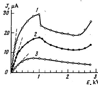
FIG. 2. Current-voltage characteristics of photocurrent  $J$  following illumination with "white" light with intensities  $I/I_0$  equal to 1.0, 0.5, and 0.25 (curves 1, 2, and 3, respectively). Sample CdCr<sub>2</sub>Se<sub>4</sub> (0.037% Ga).
