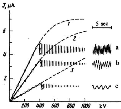
FIG. 3. Current-voltage characteristics of the photocurrent  $J$  following illumination with "white" light (dashed curve) and monochromatic light (solid curve) of intensity  $I/I_0$  equal to 0.25 (curve 1), 0.125 (curve 2), and 0.05 (curve 3). The dashed sections correspond to regions of self-oscillations of the photocurrent (a, b, c).
