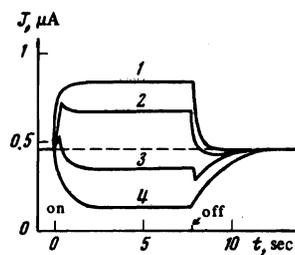
FIG. 5. Time dependences of the photocurrent  $J$  following turning on and off light with wavelengths  $\lambda = 8800, 8950, 9100,$  and  $9300$  Å (curves 1, 2, 3, and 4, respectively) at a constant background illumination  $\lambda = 8800$  Å.
