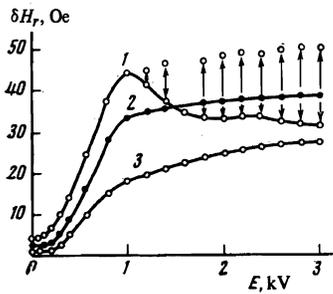
FIG. 1. Dependence of the change of the FMR field on the electric field at light intensities  $I/I_0$  equal to 1.0, 0.5, and 0.25 (curves 1, 2, and 3, respectively), with  $I_0 \sim 10^{-2}$  W/cm<sup>2</sup>. The sample is CdCr<sub>2</sub>Se<sub>4</sub> (0.037% Ga),  $T=77$  K (the arrows between the points correspond to the change of the resonant field in the instability region).
