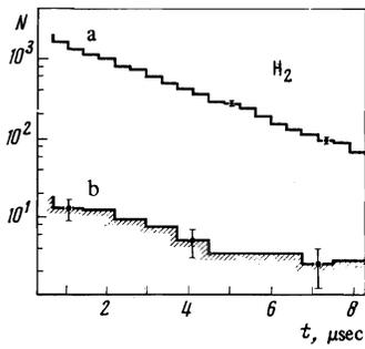
FIG. 4. Time spectra of events recorded by the detectors in coincidence with counter 5 ( $e+5$ ): a—run I, b—data of run IV normalized to number of muon stoppings in run I ( $N$  is the number of events in a  $0.378\text{-}\mu\text{sec}$  interval).
