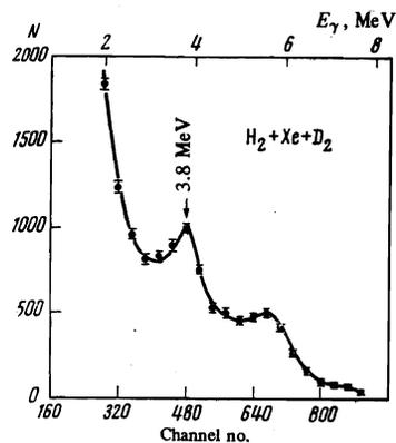
FIG. 10. Pulse-height distribution of events recorded by the  $\gamma$  detectors in run III in anticoincidence with detector 5 (the abscissa is the  $\gamma$ -ray energy and the ordinate is the number of events per 0.294-MeV interval). The energy of the  $K_\alpha$  line of mesic x rays for xenon is 3.8 MeV (the arrow indicates the location of the corresponding photopeak).
