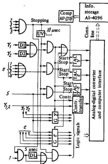
FIG. 3. Block diagram of electronics.
