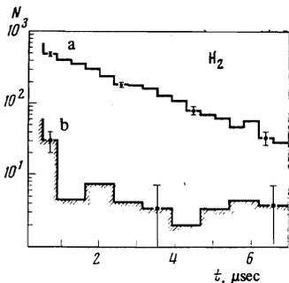
FIG. 5. Time spectra of events recorded by the  $\gamma$  detectors in coincidence with counter 5 ( $\gamma+5$ ): a—run I, b—normalized data of run IV.
