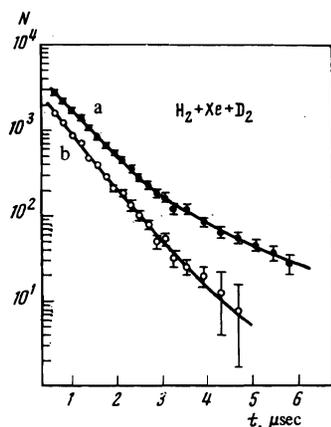
FIG. 9. Time spectra of events recorded by the  $\gamma$  detectors in run III (the normalized background has been subtracted): a—coincidences with counter 5 ( $\gamma+5$ ), b—anticoincidences with counter 5 ( $\gamma-5$ ).
