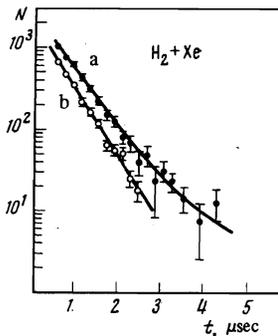
FIG. 7. Time spectra of events recorded by the  $\gamma$  detectors in run II (The normalized background has been subtracted): a—coincidences with detector 5 ( $\gamma+5$ ), b—anticoincidences with detector 5 ( $\gamma-5$ ); the solid lines are theoretical curves.
