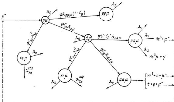
FIG. 1. Schematic diagram of processes occurring on stopping of  $\mu^-$  mesons in a gas mixture H<sub>2</sub> + Xe + D<sub>2</sub>.
