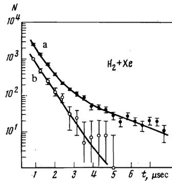
FIG. 6. Time spectra of events recorded by the  $e$  detectors in run II (the normalized background has been subtracted): a—coincidences with detector 5 ( $e+5$ ), b—anticoincidences with detector 5 ( $e-5$ ); the solid lines are theoretical curves.
