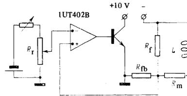
FIG. 1. Block diagram of the power supply of a solenoid  $L$ , including a storage battery of 10 V, a composite transistor, a 1UT402B feedback amplifier, a feedback resistor  $R_{fb}$ , a filter resistor  $R_f$ , a measuring resistor  $R_m$ , and a control rheostat  $R_r$ .
