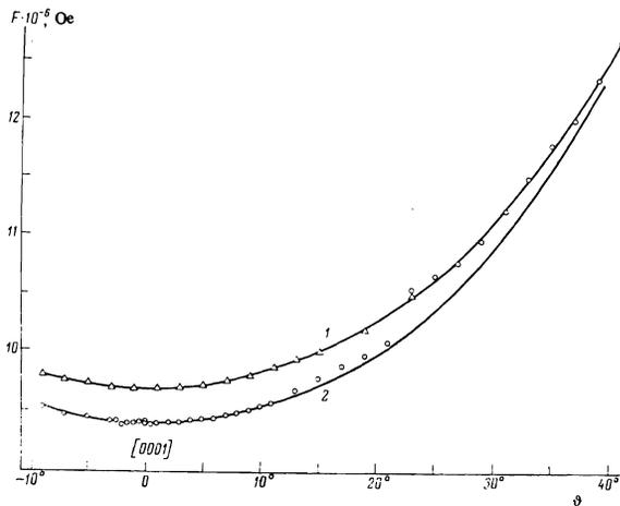
FIG. 2. Dependences of the magnetic frequency  $F$  on the angle  $\varphi$  between  $H$  and  $C$ . The continuous lines represent the dependences  $F(\varphi)$  for noncentral (1) and central (2) sections determined on the basis of the de Haas-van Alphen effect; the triangles are used to denote several control points and the circles are the results of measurements of the magnetoresistance oscillations.
