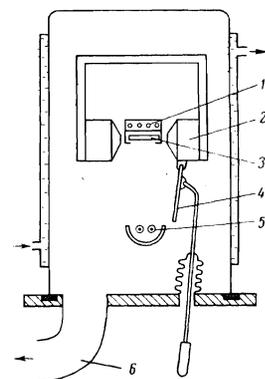
FIG. 3. Apparatus for vacuum sputtering: 1—heater, 2—magnet, 3—backing, 4—shutter, 5—tungsten spiral, 6—exhaust pipe.
