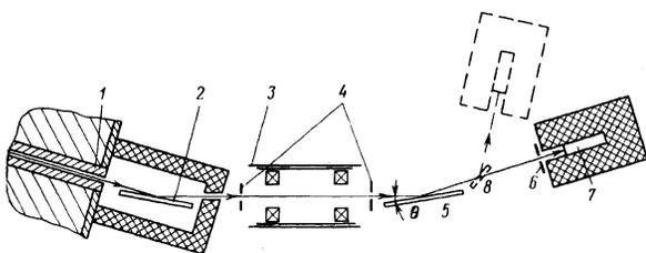
FIG. 4. Diagram of the apparatus for testing polarizing mirrors: 1—collimator, 2—polarizing mirror, 3—spin-flipper, 4, 6—cadmium slits, 5—analyzing mirror, 7— $^{10}\text{BF}_3$  detector, 8—crystal-monochromator of the spectrometer.
