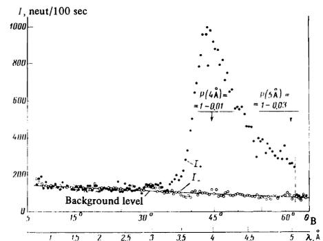
FIG. 7. Dependence of the reflection of the parallel ( $I_+$ ) and the anti-parallel ( $I_-$ ) components of the beam on the neutron wavelength  $\lambda$  for a 50Fe50Co mirror with a 85Ti15Gd substratum.  $\theta_B$  is the Bragg angle for the analyzing (111) plane of a single crystal of Pb.
