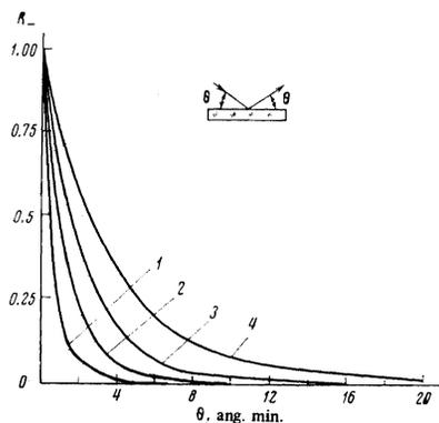
FIG. 2. Calculated dependence of the reflection coefficient  $R$  on the glancing angle  $\theta$  for a 50Fe50Co alloy: curve 1— $\lambda=3$  Å, 2— $\lambda=6$  Å, 3— $\lambda=10$  Å and for Ti: curve 4— $\lambda=6$  Å.
