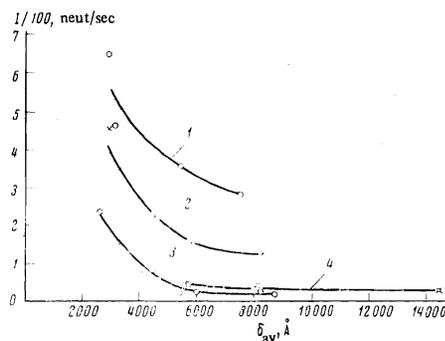
FIG. 5. Dependence of the intensity  $I$  of beams reflected at a glancing angle of  $\theta = 21'$ , on the thickness of the film for Ti-Gd mirrors of different compositions: 1—98Ti2Gd, 2—95Ti5Gd, 3—85Ti15Gd, 4—60Ti40Gd.
