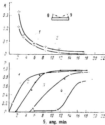
FIG. 6. a) Dependence of the reflection coefficient on the glancing angle: 1—for a 60Ti40Gd mirror, 2—for a 85Ti15Gd mirror. b) Dependence of the polarizing ability on the glancing angle. Composition of the ferromagnetic layer with a 85Ti15Gd substratum: 1—40Fe60Co, 2—50Fe50Co, 3—54Fe46Co and without a substratum: 4—50Fe50Co.
