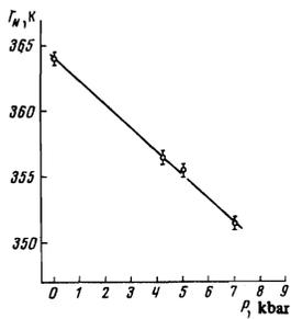
FIG. 6. Pressure dependence of the effective magnetic field at the  $\text{Fe}^{57}$  nuclei in  $\text{FeF}_3$ .
