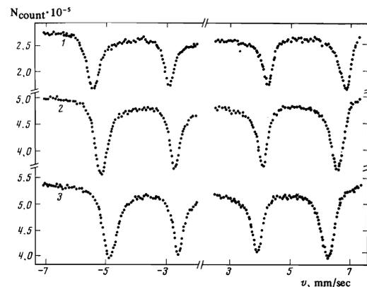
FIG. 5. Mössbauer spectra of Fe<sup>57</sup> nuclei in FeF<sub>3</sub>: 1)  $P = 1$  atm, 2)  $P = 5$  kbar, 3)  $P = 10$  kbar.
