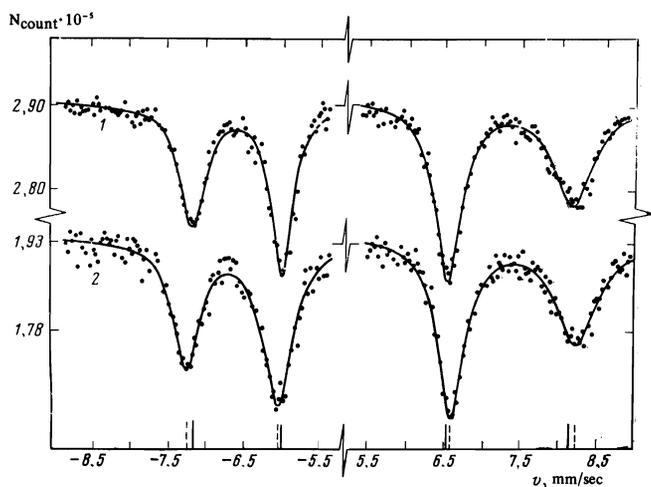
FIG. 1. Mössbauer spectra of  $\text{Fe}^{57}$  nuclei in  $\text{Y}_3\text{Fe}_5\text{O}_{12}$  (outer peaks of two sextets): 1)  $P = 1$  atm, 2)  $P = 14$  kbar,  $N_{\text{count}}$ —number of counts.
