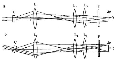
FIG. 1. Experimental setup. a—laser beam propagates along the optical axis Y of the spectrograph and is incident perpendicular to the (010) surface of the crystal C;  $L_1$ ,  $L_2$ ,  $L_3$ —lenses, F—filter, Sp—spectrograph slit (the Z axis is in the plane of the figure); b—laser beam directed at an angle to the optical axis.
