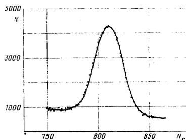
Section of experimental neutron-diffraction curve of TbAg in the region of the reflection (110)M, obtained at temperature  $0.05^\circ\text{K}$ ;  $N_c$  is the number of the analyzer channel of  $40 \mu\text{sec}$  width and  $N$  is the number of the detector counts.
