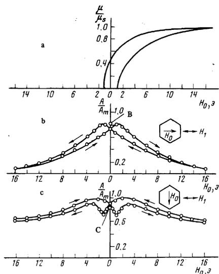
FIG. 1. Hysteresis loop (a) and dependence of the relative amplitude of the spin echo on the field for  $H_0 \parallel H_1$  (Fig. b) and for  $H_0 \perp H_1$  (c) for the reversal of the magnetization of single-crystal FeBO<sub>3</sub>.  $A_m$  is the maximum echo amplitude.
