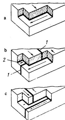
FIG. 2. Schematic model of reversal of FeBO<sub>3</sub> magnetization. The arrows show the direction of the magnetization in the domain. In Fig. b, 1 and 2 are the Neel and Bloch walls, respectively.
